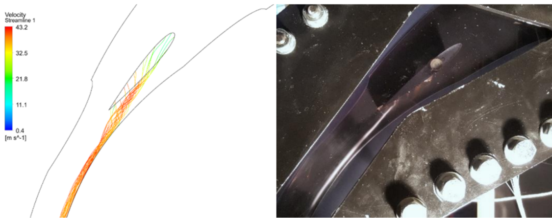
Figure 4.16: Vortex from the clearance gap (side view)
