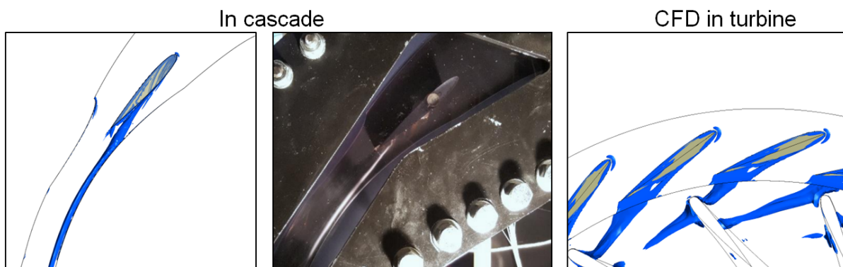
Figure 6.4: Vortex filament observed from CFD and experiment
