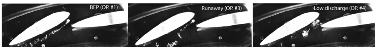
Figure 3.4: Vortex formations around guide vanes at different operating conditions [33]
