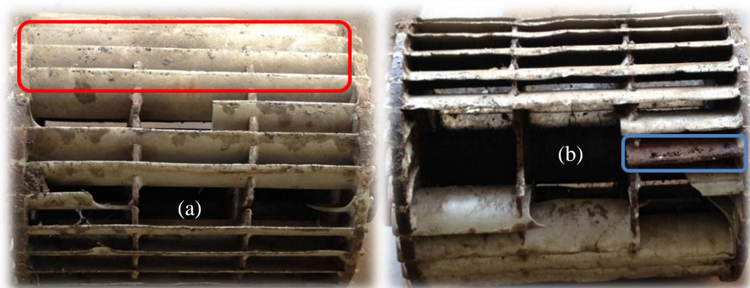
Figure 1-1: Damaged CFT (a) runner 1 and (b) runner 2 of Daran Khola MHP due to sediment erosion
