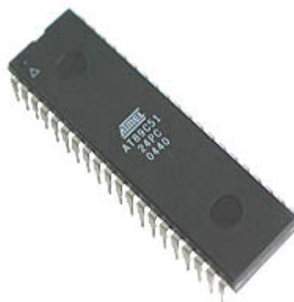
Figure 1.2: 8051 and 8052 family microcontrollers (Prachi Dukale, 2019)
