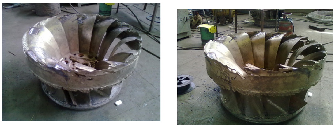
Figure 1.1: Effect of sediment erosion in Francis turbine
