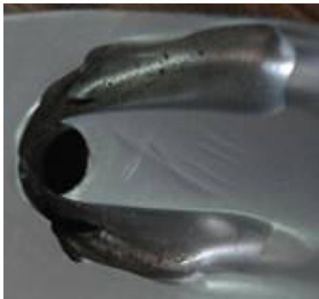
Figure 2.6: Erosion pattern generated by sand erosion [52].
