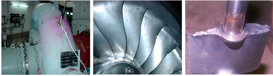
(a) Locations of sensors. (b) Runner condition during experiment. (c) Guide vane eroded condition.
