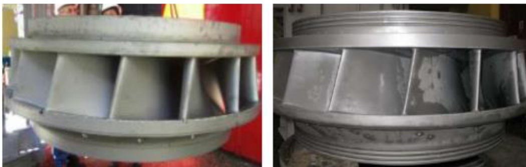
Figure 2.15: Pilot runner after 130,000 tons of sediment load (left) and Phase 2 runner after 159,000 tons of sediment load (right) [52].
