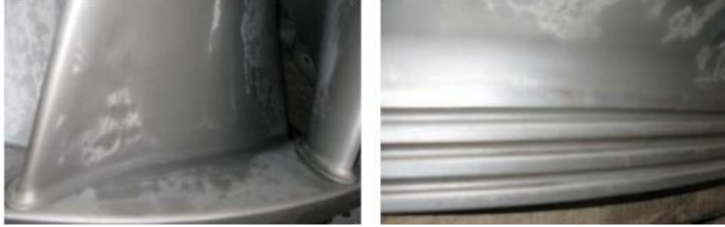
Figure 2.16: Joint between runner blade and hub after 159,000 tons of sediment load (left) and Edge of labyrinth seals after 159,000 tons of sediment load (right) [52].
