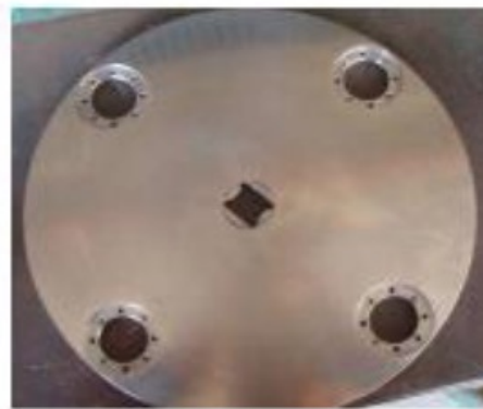
b) Rotating disc with 4 locations for test specimens
