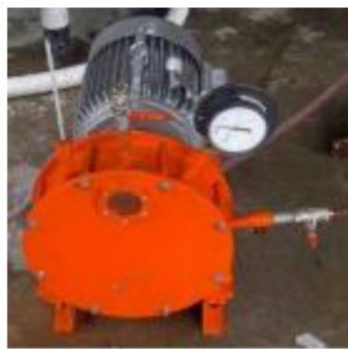
a) Setup for testing erosion on joints
